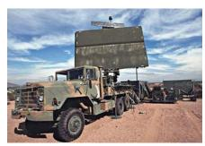
The AN/TPS-75 is a mobile, tactical radar system capable of providing radar azimuth, range, height and Identification Friend or Foe (IFF) information for a 240 nautical-mile area. It is a deployable/transportable radar system capable of providing long range radar data to support operations and control of tactical aircraft. It forms the backbone of the US Air Force Air Defense
